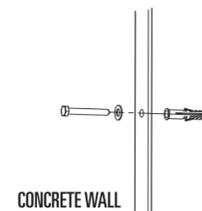
**CAUTION: THE FAN IS ONLY SUITABLE FOR CONCRETE WALL AND WALL STUD. DO NOT USE FOR DRY WALL MOUNTING. USE THE MOUNTING ACCESSORIES SHIPPED WITH PRODUCTS FOR WALL MOUNTING.**
